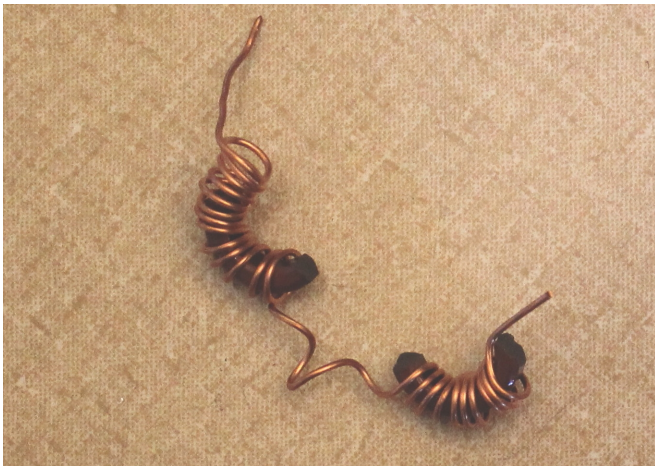
Figure 5. Toroid with hard-drawn copper wire.
