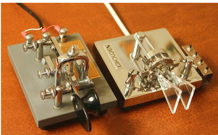
Figure 5. A single-lever paddle for use with an electronic keyer is shown at left. The double-paddle key at right is also suitable for iambic keying.
